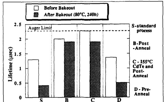
Fig. 4. Minority carrier lifetime of  $n = 1 \times 10^{15} \text{ cm}^{-3}$  LPE grown HgCdTe layers passivated with thermally evaporated CdTe before and after bakeout at 80°C for 240 h.
