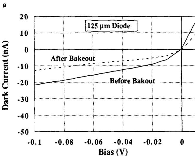
Fig. 2. (a) Standard process sequence. Dark current I-V curves before and after 240 h bakeout for 22  $\mu\text{m}$  (mesa-size) diode, and (b) dark current I-V curves before and after 240 h bakeout for 125  $\mu\text{m}$  (mesa-size) diode.
