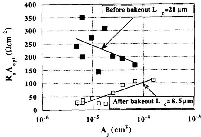
Fig. 5. Standard process sequence.  $R_o A_{opt}$  performance as a function of detector junction area before and after bakeout for 240 h at 80°C.
