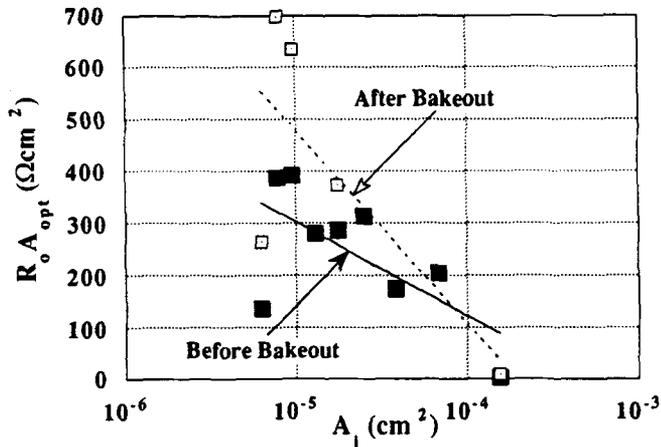
Fig. 9. CdTe deposited at 155°C followed by a Hg anneal.  $R_0A_{opt}$  performance as a function of detector junction area before and after bakeout for 240 h at 80°C.
