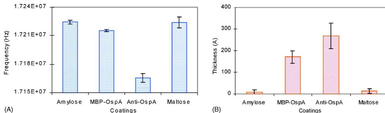
Fig. 7.  $\mu$ CANARY resonant frequency response (A) and ellipsometry measurements (B) for detection of anti-OspA antibody. With the immobilization of each coating, more mass was added to the sensor, which induced the decrease in frequency signal and the increase in coating thickness on the sensor surface. When maltose was added to the sensor after detection, the sensor surface was re-generated. Error bars represent the standard deviation of five measurements.
