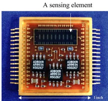
Fig. 3. Photo of a multiple-element  $\mu$ CANARY sensor package.
