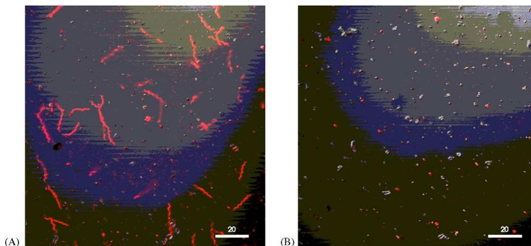
Fig. 9. Confocal microscopy pictures for  $\mu$ CANARY sensors that have anti-OspA coated on the surface and have been exposed to *Borrelia* N40 (A, Nile-red labeled spirochet, with OspA on outer coat) and *Borrelia* 7  $\times$  297 (B, without OspA on outer coat), respectively. The scale shown in the pictures is 20  $\mu$ m. The frequency shifts observed for A and B are  $\sim$ 27 and  $\sim$ 4 kHz, respectively.
