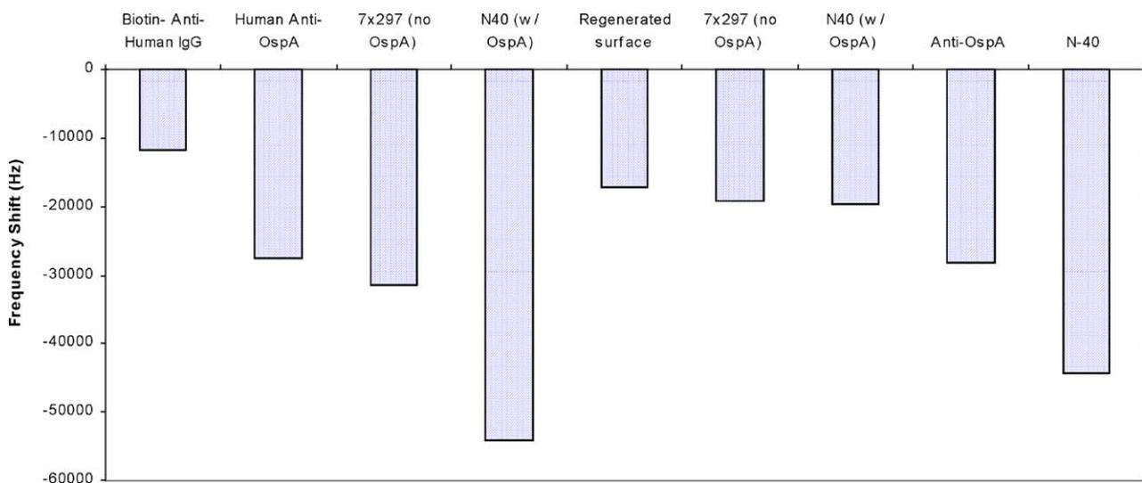
Fig. 8. Preparation of  $\mu$ CANARY sensor with affinity ligand protein anti-OspA for detection of wild-type *B. burgdorferi* (strain N40) expressing OspA on its outer surface. Mutant strain 7  $\times$  297, which does not express OspA, is not detected. The sensor surface is subsequently stripped of anti-OspA using pH shock. The sensor without anti-OspA detects neither N40 nor 7  $\times$  297. When anti-OspA is immobilized on the sensor, it again detects the N40 strain.
