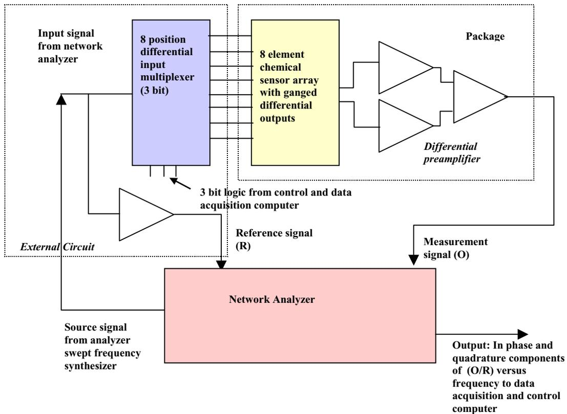
Fig. 2. Schematic of circuitry for 8-element  $\mu$ CANARY sensor in open-loop measurement.
