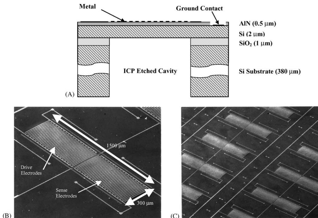
Fig. 1. (A) Cross-section diagram of the FPW resonating membrane structure, (B) SEM photo of a sensor element from the top surface of the wafer showing detail of metal electrode structure, and (C) SEM photo of several integrated FPW membranes within a section of an integrated sensor array.
