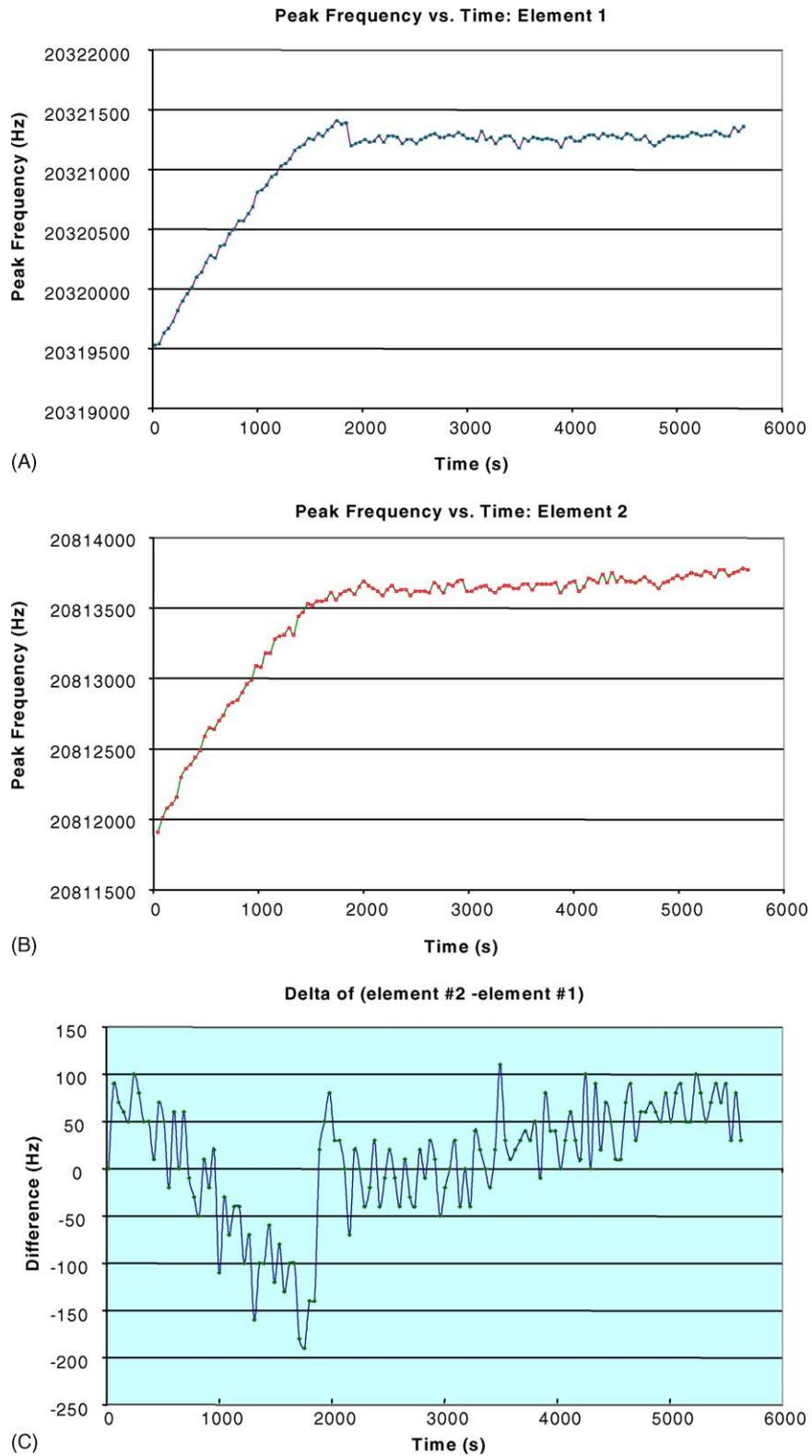
Fig. 4. Resonance frequency readings in air of two elements on a multi-sensor array over a 100 min period. (A) Peak frequency reading for element 1; (B) peak frequency reading for element 2; (C) peak frequency reading difference between elements 2 and 1.
