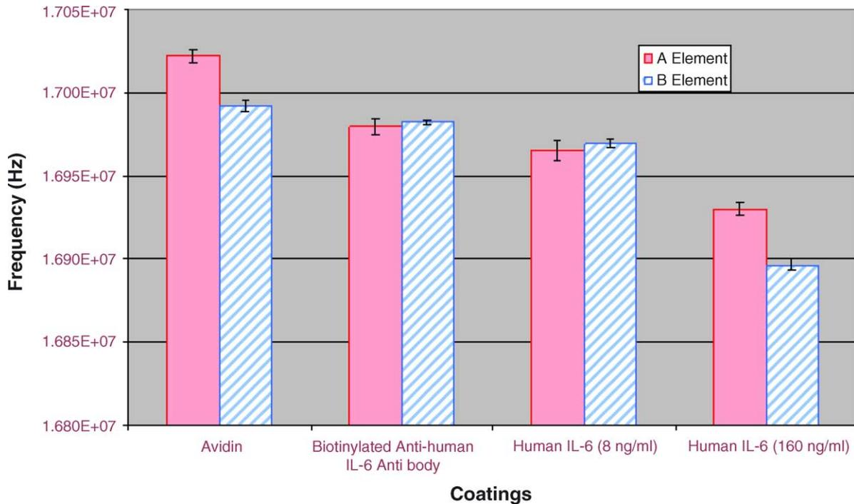
Fig. 6. Frequency response of two sensing elements (A and B) within a 2-element  $\mu$ CANARY to recombinant human interleukin-6. The frequencies shown are the average value of 10 readings. In the experiment, conditions were not optimized to determine the sensitivity of the sensor response. Estimate of the sensitivity was made based on the relative signal level above experimental noise.
