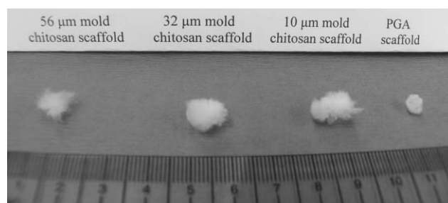
Fig. 8 Size of the lyophilized chitosan scaffolds with non-woven polyglycolic acid (PGA) fibers as a reference, relative to a scale in centimetres. The dry weight of all are standardized to approximately 2 mg.
