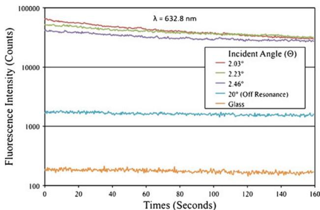
**Fig. 5** Plot of the measured fluorescence intensity versus time for continuous exposure at different angles of incidence for the excitation light
