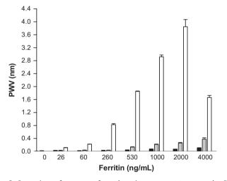
**Fig. 2.** Comparison of responses from three immunoassay types on the PC biosensor for different ferritin standard concentrations in PBS buffer. Label-free assay (black bars); sandwich assay with secondary antibody (gray bars); immuno-functionalized IONPs with secondary antibodies (white bars). Bars represent mean  $\pm$  SD (n=3, average of separate assays).
