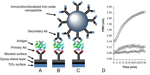
**Fig. 1.** A schematic of the three immunoassay types on the PC biosensor and their real-time kinetic readings for ferritin  $(1 \ \mu g/mL)$  in the BIND system. (A) label-free assay; (B) with secondary antibody sandwich assay; (C) immunofunctionalized IONPs with secondary antibodies; (D) kinetic readings: label-free assay ( $\diamond$ ), with secondary antibody sandwich assay ( $\Box$ ), and immunofunctionalized IONPs with secondary antibodies ( $\circ$ ).
