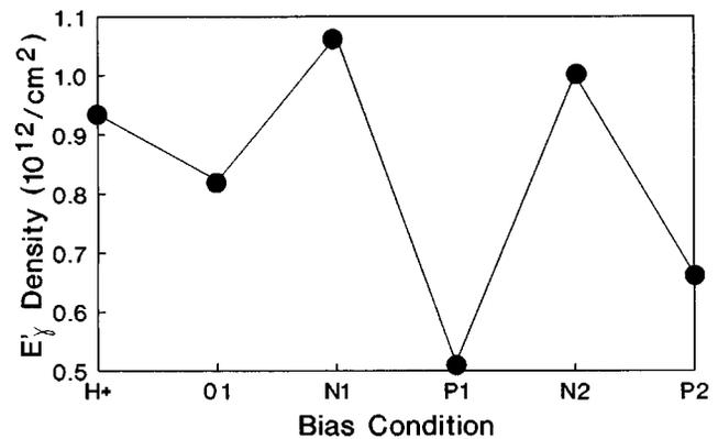
FIG. 2.  $E'_\gamma$  density vs various 24 h bias sequences.
