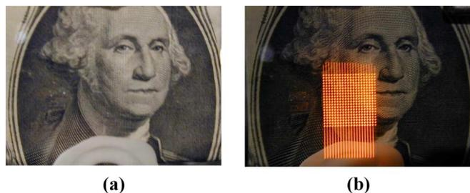
Fig. 4. Photograph of a  $20 \times 20$  array of microplasma cavities situated between a U.S. one dollar bill and the camera: (a) the image before ignition of the array and (b) CCD image with device operated at a Ne pressure of 700 torr and an rms voltage of 340 V.
